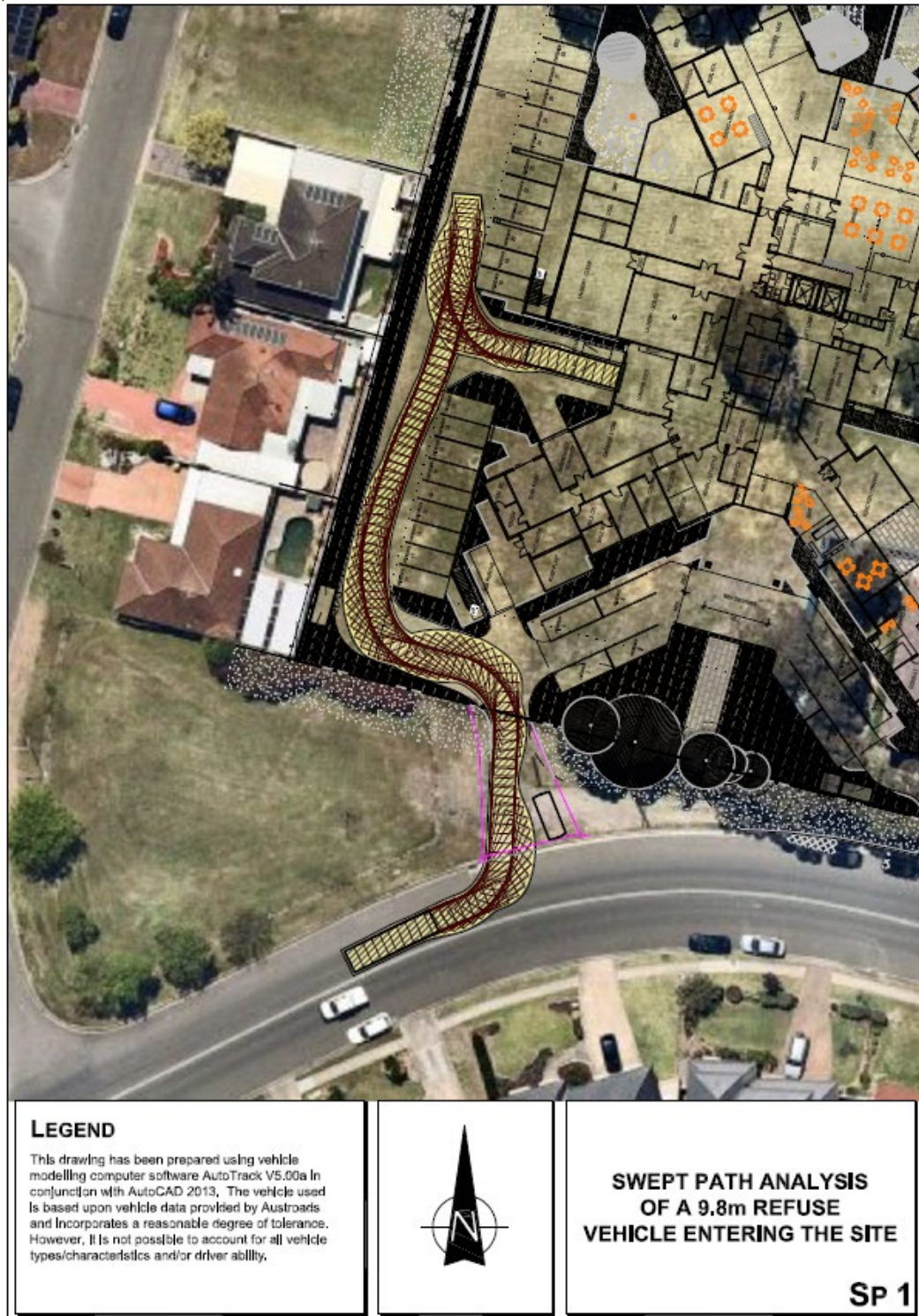
Figure 6 Vehicle entering Swept Path details provided by the Traffic Consultant.
